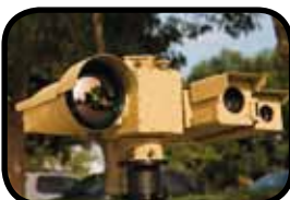
WALRSS integrated onto NightHawk EO/IR Surveillance System
